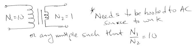
2. [3 PTS] The transformer above is hooked to a 9 volt battery. What are the possible output voltages?
